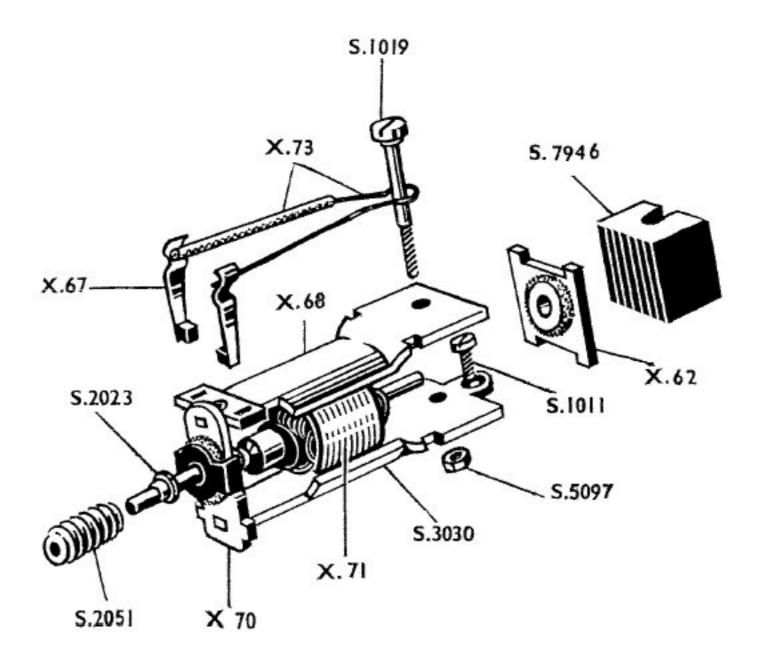
X.62 Back Plate and Bearing X.67 Brush Arm and Brush X.68 Top Pole Piece with Diaphragm X.69 Diaphragm and eyelet (Shown as part of X.68) X.70 Front Plate and Bearing X.71 Armature and Commutator X.73 Brush Spring and Insulator S.1011 Motor Securing Screw 5.1019 Magnet Screw 5.2023 Thrust Bush S.2051 Two Start Worm Bottom Pole Piece 5.3030 S.5097 Magnet Nut S.7946 Magnet
